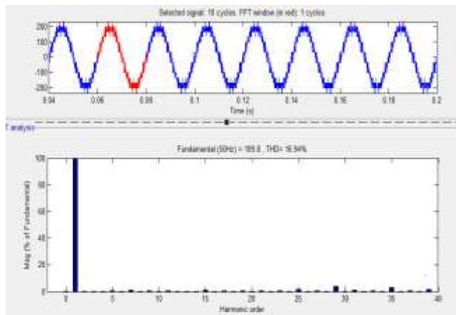
Fig. 10. Harmonic spectrum of output voltage waveform for Three-Phase Five-Level Inverter for R-Phase.
