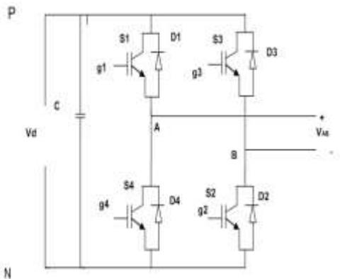
Fig. 1. Basic Three-level Inverter.
