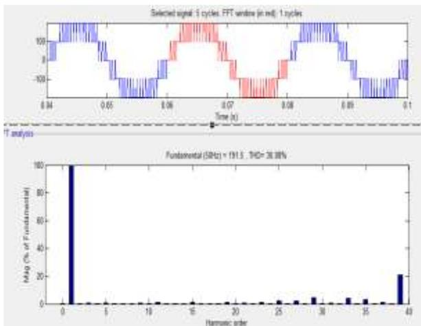
Fig. 8. Harmonic spectrum of output voltage waveform for Single-Phase Five-Level Inverter.
