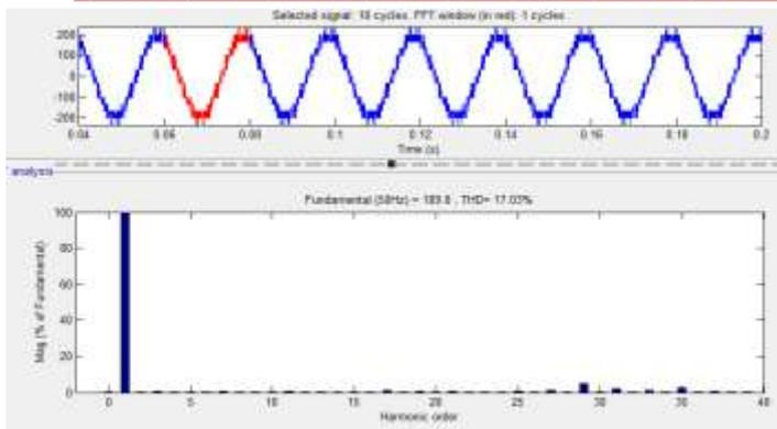
Fig. 12. Harmonic spectrum of output voltage waveform for Three-Phase Five-Level Inverter for B-Phase.
