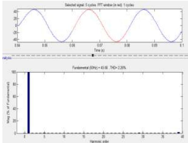
Fig. 9. Harmonic spectrum of output current waveform for Single-Phase Five-Level Inverter.
