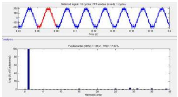
Fig. 11. Harmonic spectrum of output voltage waveform for Three-Phase Five-Level Inverter for Y-Phase.
