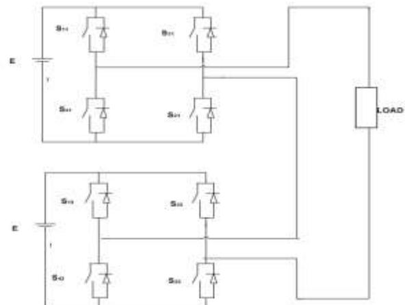
Fig. 2. Five-Level Inverter with Equal dc voltage
