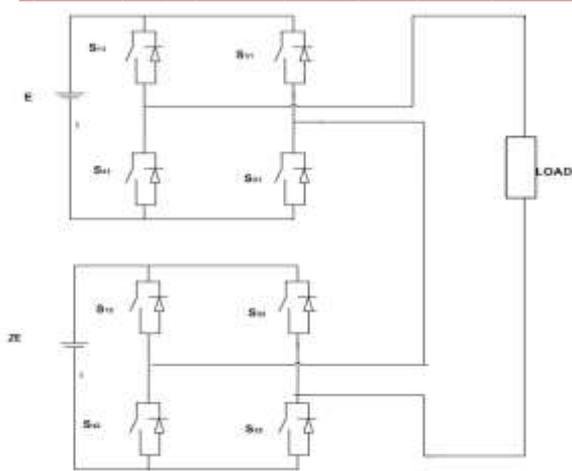
Fig. 3. Per - phase diagram of CHB with Unequal dc voltage
