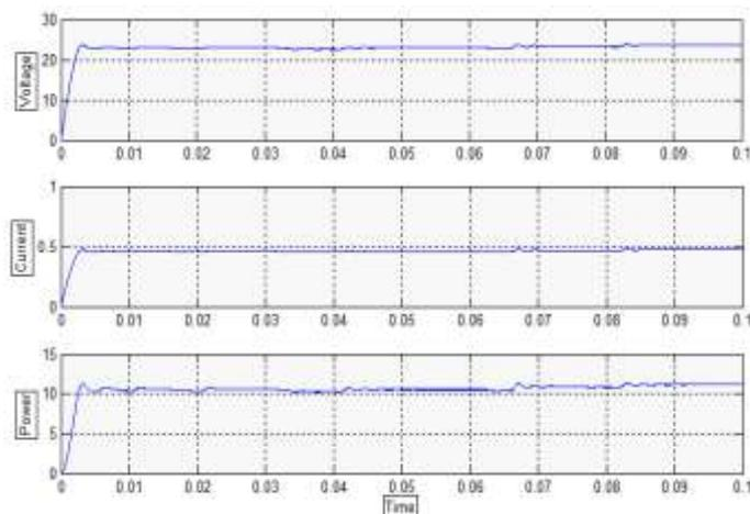
Figure 13: Output Voltage, Current and Power waveform at different G and constant  $T_{op}=25^{\circ}C$ .
