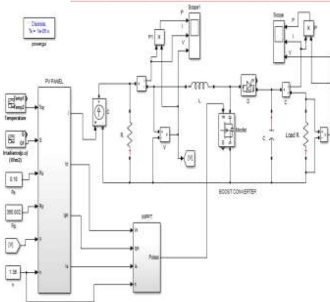
Figure 6: Matlab Model of Tracking System
