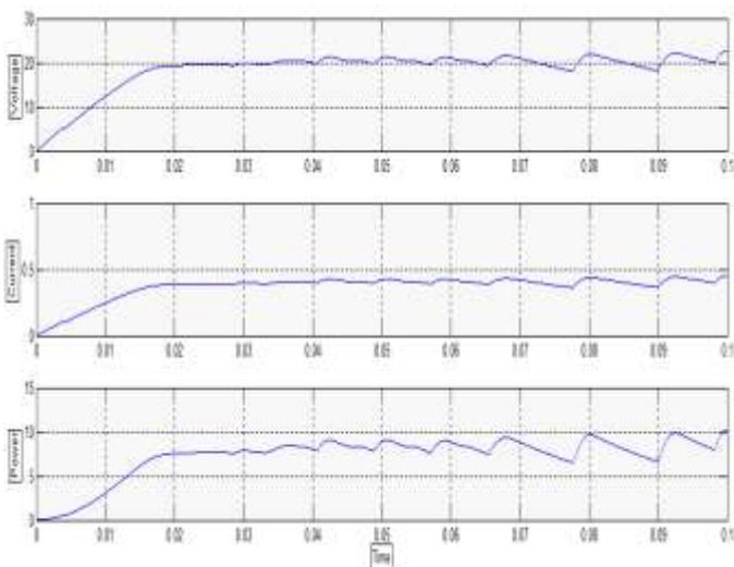
Figure 7: Output Voltage, Current and Power waveform at different G and constant  $T_{op}=25^{\circ}C$ .
