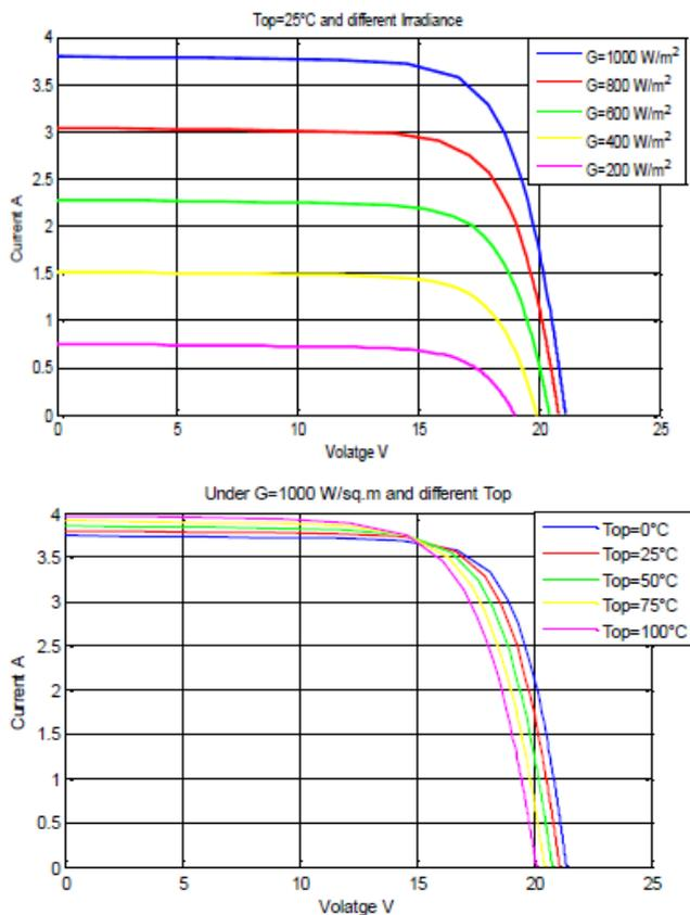
Figure 3: I-V characteristics at different G and Top
