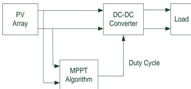
Figure 1- Block Diagram of Tracking System
