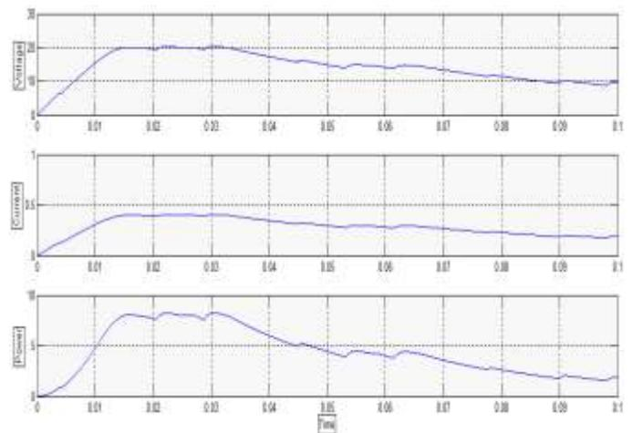
Figure 8: Output Voltage, Current and Power waveform at different  $T_{op}$  and constant  $G=1000 W/m^2$ .
