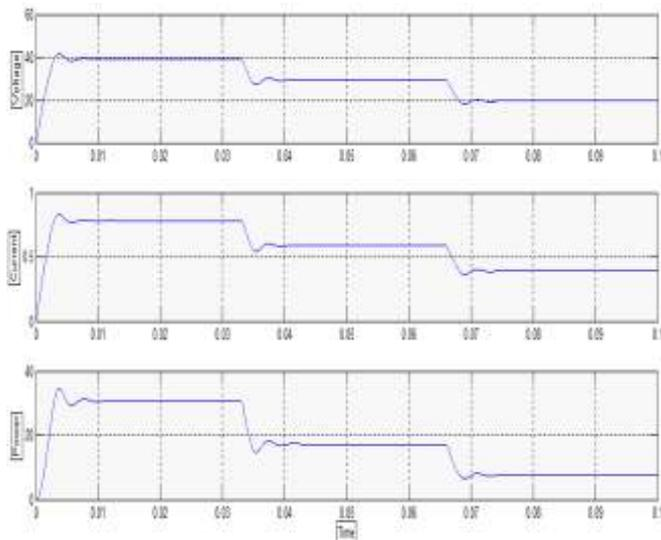
Figure 12: Output Voltage, Current and Power waveform at different  $T_{op}$  and constant  $G=1000 W/m^2$ .
