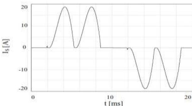
Figure.2 Diode bridge rectifier front-end ASD system (5.5kW) (a): Line current waveform
