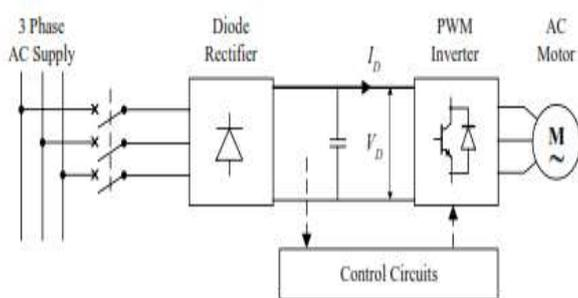
Figure.1 Variable Frequency Drive
