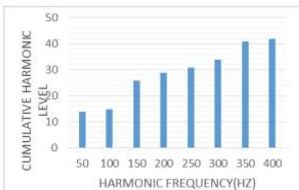
Figure.6: Harmonic levels at VFD
