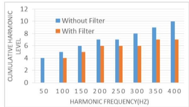
Figure.7: Harmonic levels at PLC without and with filter
