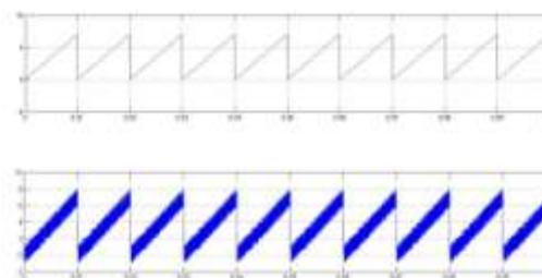
Figure 6(c): Response to Ramp wave
