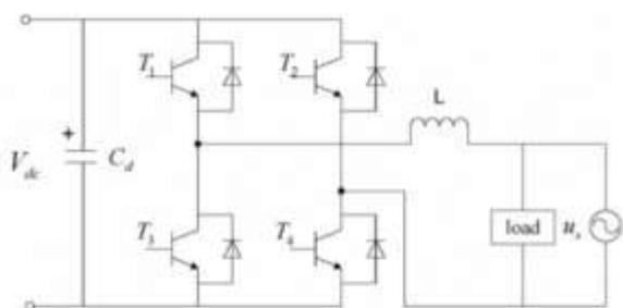
Figure 1: Structure of Grid Connected Inverter
