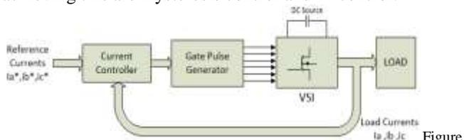
Figure 2: Functional Block diagram of Current Controlled PWM Inverter
