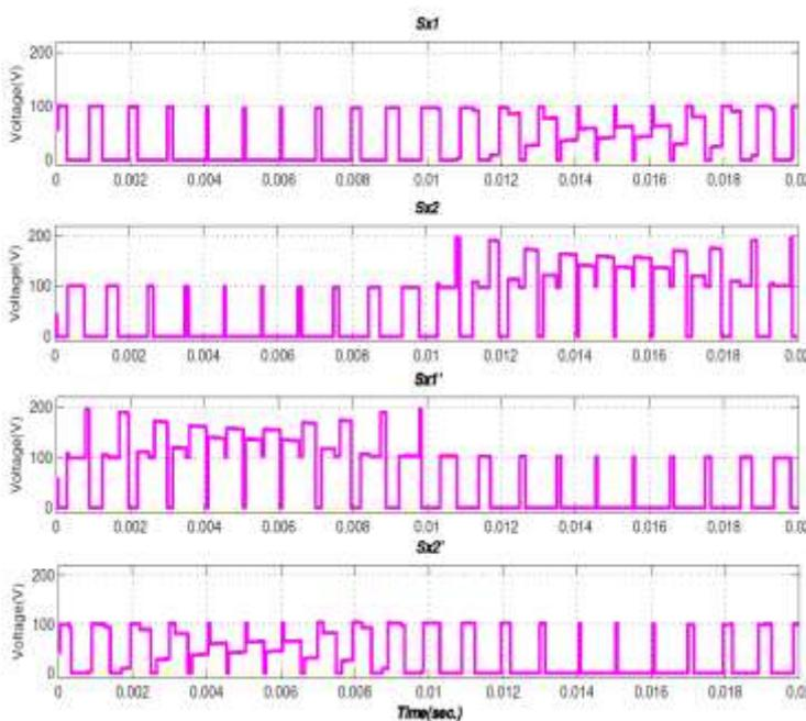
Figure 4(a) Voltage across Switch in 3L-NPC with PS-PWM
