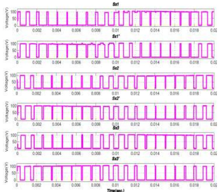
Figure 4(b) Voltage across Switch in 3L-ANPC with PS-PWM
