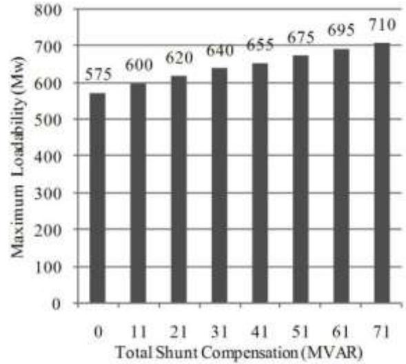
Figure 4 Maximum loadability with shunt compensation
