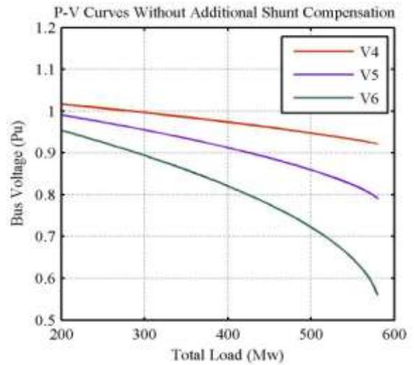
Figure 5 P-V curves without shunt compensation
