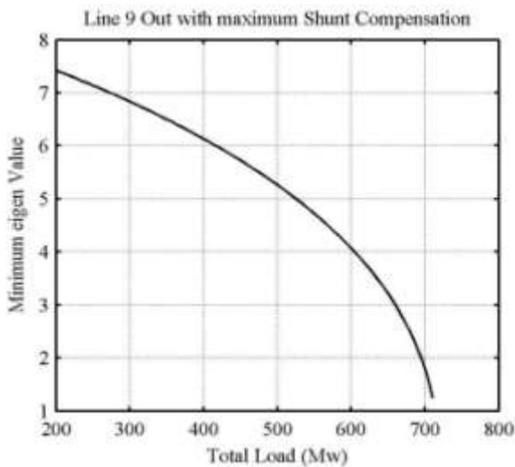
Figure 3 Variation of minimum eigen value with shunt compensation
