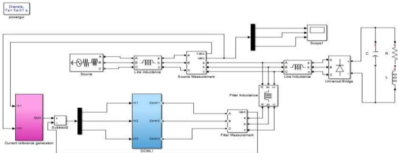
Figure 3. Overall simulation model of shunt active power filter
