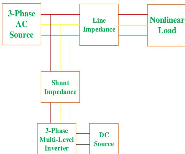
Figure 1. Shunt active power filter
