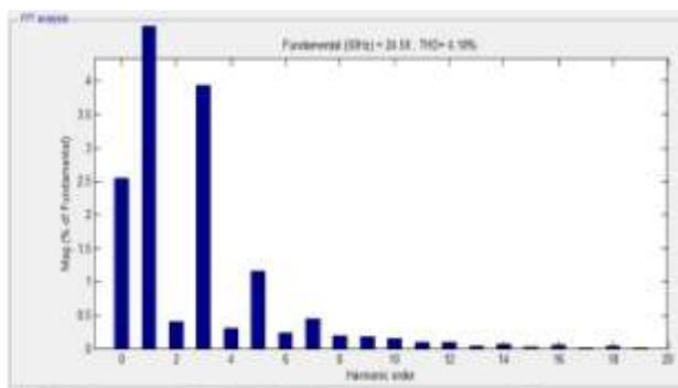
Figure 7. THD spectrum with shunt active power filter
