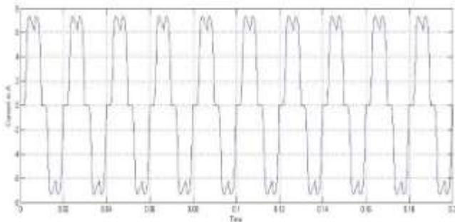
Figure 4. Source current in phase a without filter
