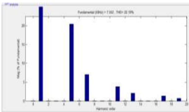
Figure 5. THD spectrum without filter
