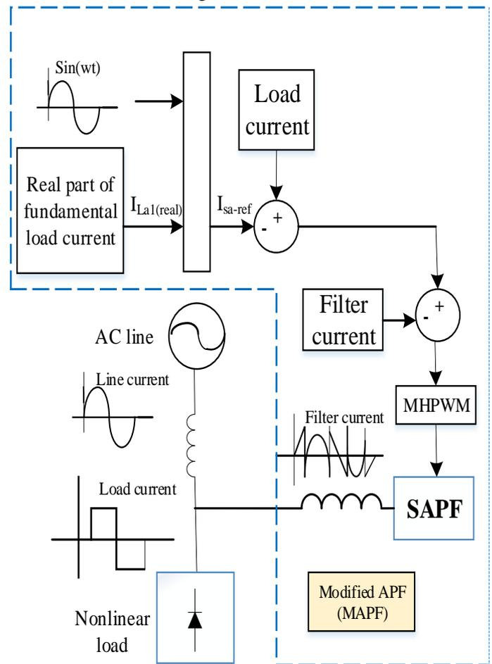
Figure 2. System overview with modified active power filter
