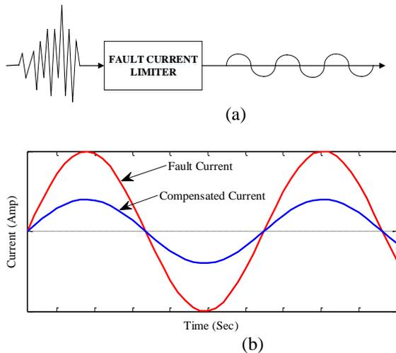
Fig. 1: (a) Fault Current Limiter Module Output(b) Fault Current Waveform and Compensated Fault Current Waveform Using SFCL
