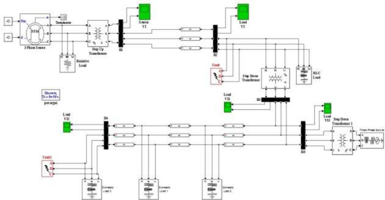
Fig. 9: Proposed System without SFCL Module
