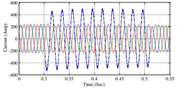
Fig. 8: Fault Current Compensated in Distribution Line with SFCL
