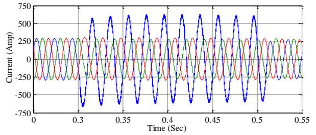
Fig. 7: Fault Current in Distribution Line without SFCL
