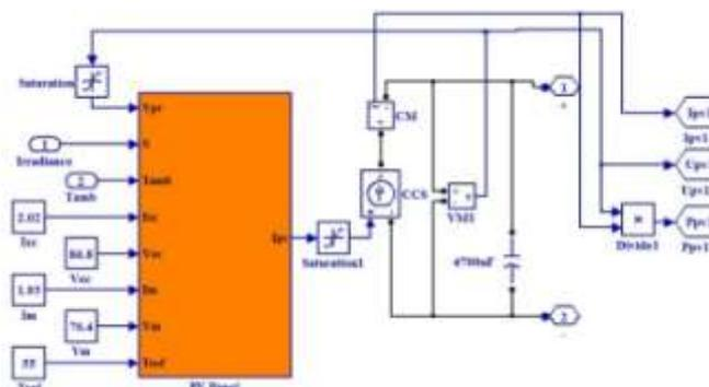
Figure 3. Simulation model of PV system
