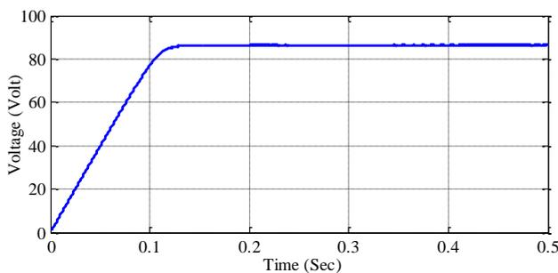
Figure 5. Common DC Link Voltage Waveform
