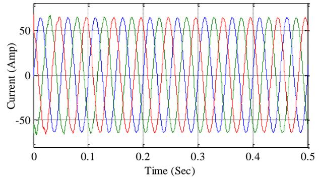
Figure 7. Grid current waveform after interconnection
