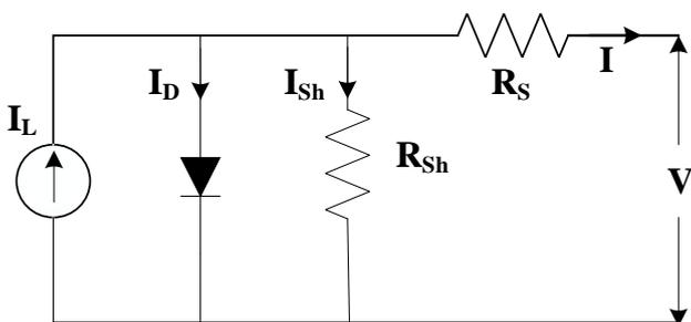
Figure 2. Photo-Voltaic model
