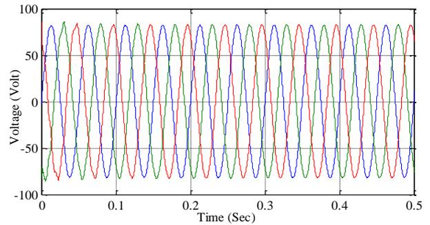
Figure 6. Grid voltage waveform after interconnection
