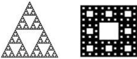
Figure 3. Some common fractal geometry found in antenna applications. Sierpinski gaskets and carpets , used in multiband antennas[ 42].
