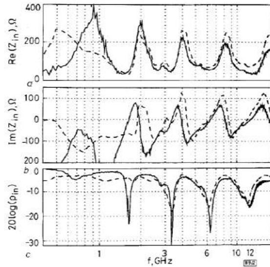
Fig. 5 . Input impedance and input reflection coefficient [42]
