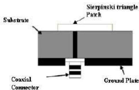
Fig. 6 Construction of Probe feeding mechanism [41]
