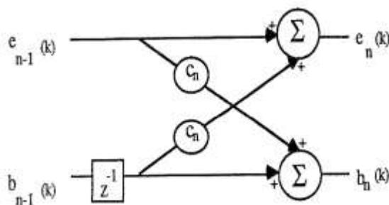
Figure:(c) Lattice Filter Structure
