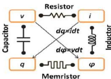
FIG.1: FOUR FUNDAMENTAL CIRCUIT ELEMENTS
