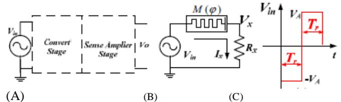
FIG.5 (A) READ OPERATION STAGES (B) CONVERT STAGE CIRCUIT (C) READ SIGNAL PATTERN [4]
