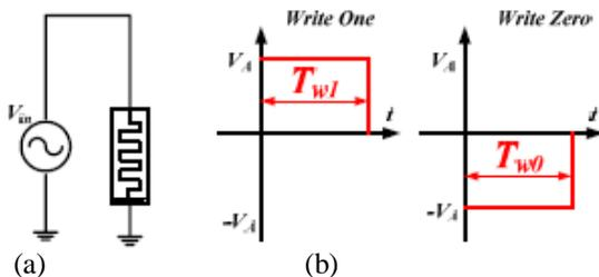
FIG.4: (A) MEMRISTOR WRITE OPERATION (B) WRITE SIGNAL PATTERNS [4]
