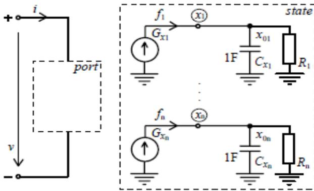
Fig. (6) General Block diagram of Spice model for  $n^{th}$  order mem-system [5]
