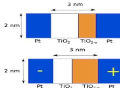
FIG.2: MEMRISTOR DEVICE STRUCTURE AND CIRCUIT MODEL
