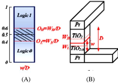
FIG.3: (A) OUTPUT LEVELS (B) MEMRISTOR 3D NANO STRUCTURE [4]
