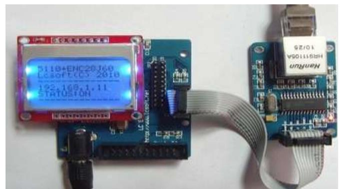
Figure 4: Ethernet Module [17]
