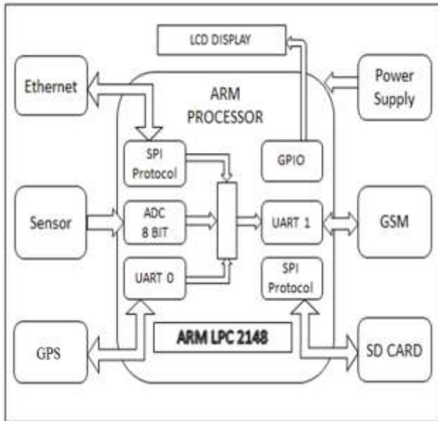
Figure 1: Block diagram of Proposed Architecture
