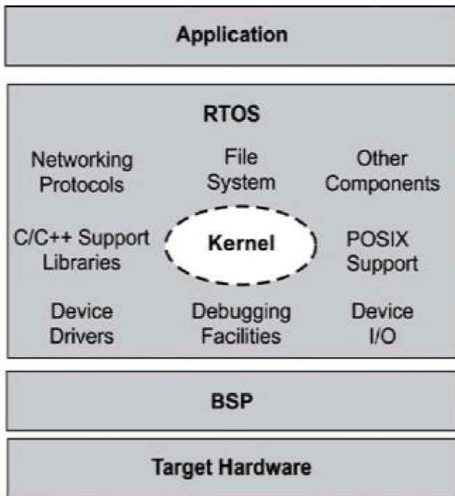
Figure 6: Hardware &  $\mu$ C/OS-II Interface[18]
