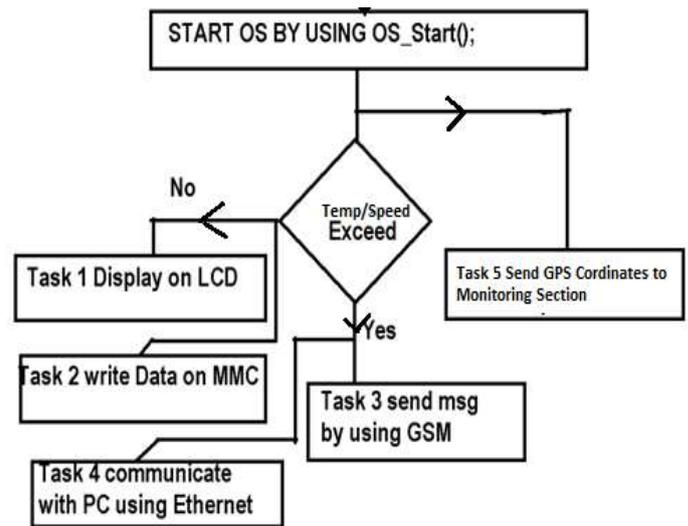
Figure 7: Flow chart of Hardware &  $\mu$ COS II Implementation
