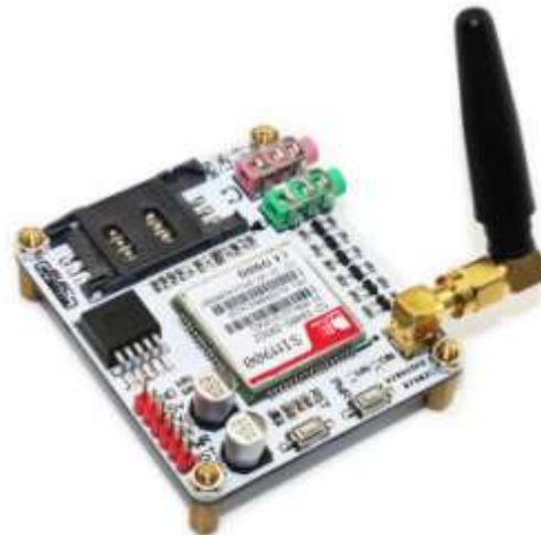
Figure 3: GSM Module [16]
