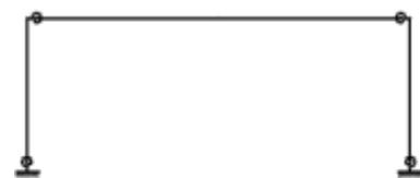
Figure 1. Semi rigid jointed frame
