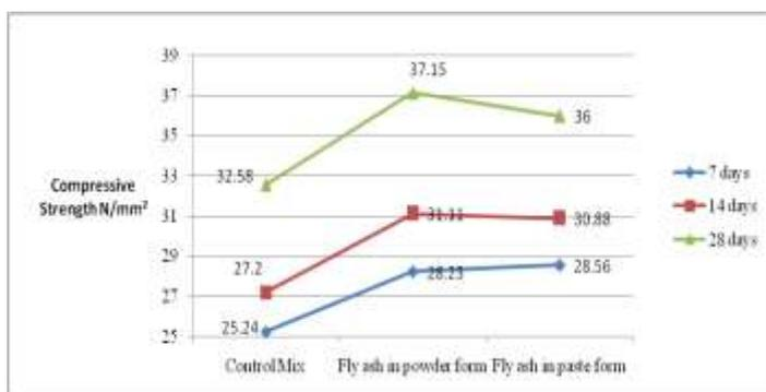
Figure 4 Compressive strength for M30 grade of concrete (Standard Concrete)
