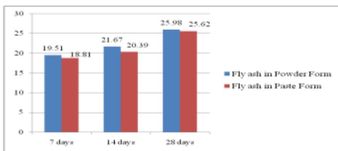
Figure. 5 Plain Comparison of Compressive strength of M20 grade of concrete with fly ash in powder and paste form
