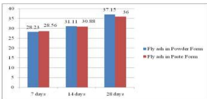
Figure 6 Plain Comparison of Compressive strength of M30 grade of concrete with fly ash in powder and paste form
