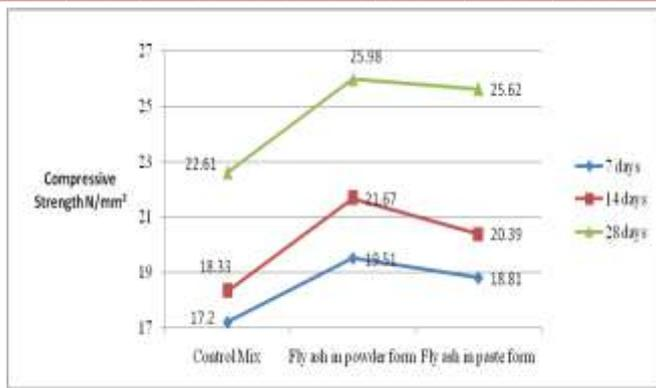
Figure. 3 Compressive strength of M20 grade of concrete
