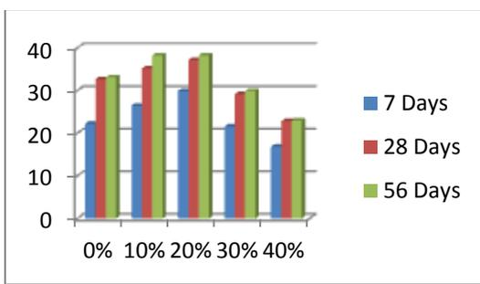
Table shows the results of **Split tensile Strength** in  $N/mm^2$  of concrete with glass powder replacement in cement in different proportions over 7, 28 and 56 days.
