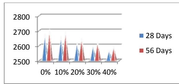
Figure-5.3 shows the results of **Ultra Sonic Pulse Velocity** in  $meter/second$  of concrete with glass powder replacement in cement in different proportions over 7, 28 and 56 days.
