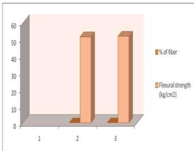
Graph 3.3 28 Days Flexural Strength (0.75% Steel fiber)
