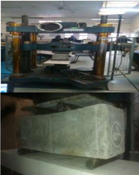
Fig 3.2 Testing of flexural strength of steel fiber reinforced Beam
