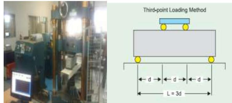
Fig No.2.1 Arrangement for Two-Point loading.
