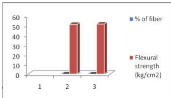
**14 Days Flexural Strength (0.75 % Steel fiber)**
