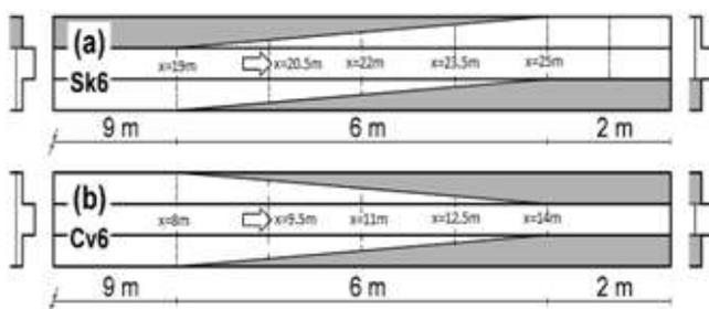
Fig 1: Configuration of the Experimental flume a) skewed b) converging
