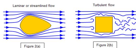
Figure 2: laminar (a) and turbulent flow (b)
