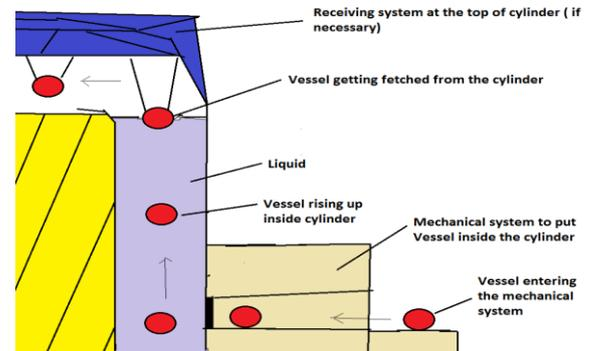
Figure3: The model: lifting of vessel by buoyancy
