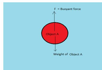
Figure 1: Buoyancy acting on a submerged object.
