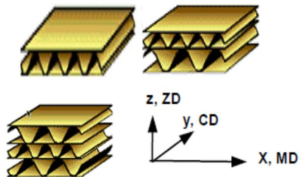
Fig. 1 Types of corrugated board a) Single wall b) Double wall c) Triple wall.
