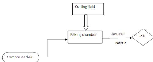
Figure 1. optimal lubricat flow system
