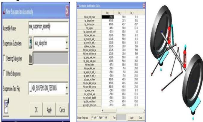
Fig 8. New Suspension Assembly and Hard point modify table Open Dialog Box In ADAMS (Car) Window
