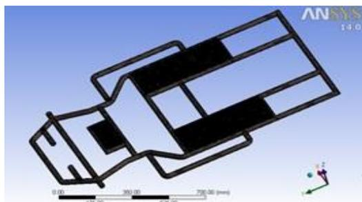
FIG.4 MESHING OF CHASSIS
