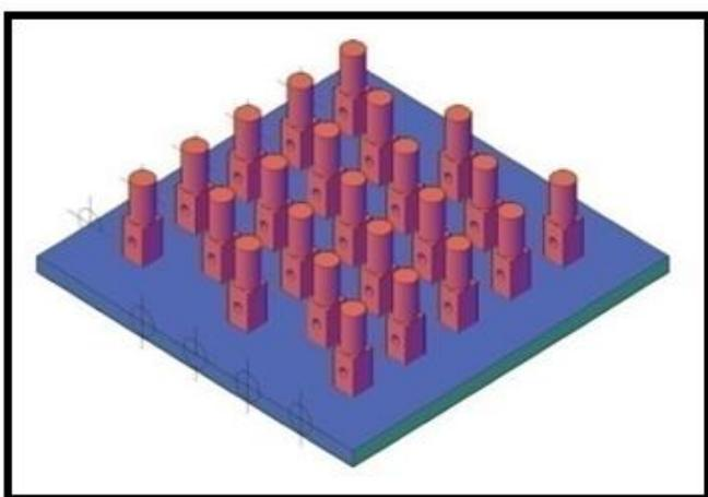
Figure 1. Base Plate of Compound Fins having bottom Square cross-section
