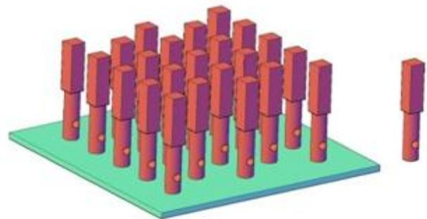
Figure 2. Base Plate of Compound Fins having bottom Circular cross-section
