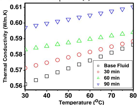
Figure 5. Variation of thermal conductivity of ZrO<sub>2</sub>/H<sub>2</sub>O nanofluids
