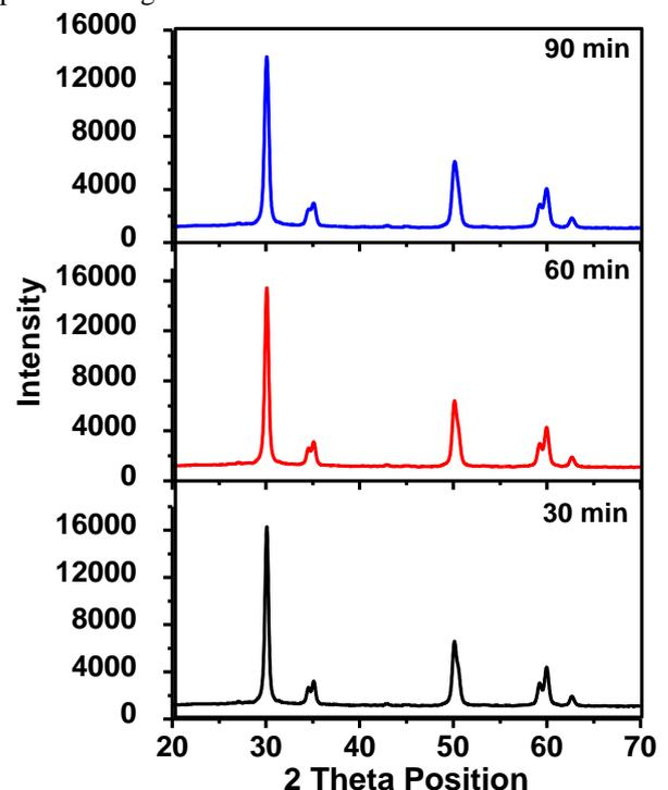
Figure.1. XRD patterns of  $ZrO_2$  nanoparticles.
