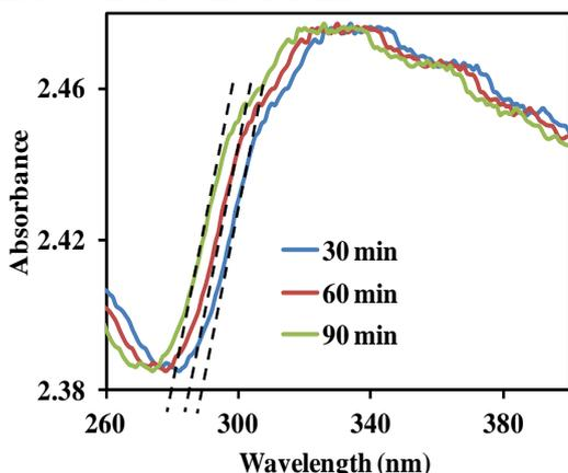
Figure 3. UV-VIS spectrum of ZrO<sub>2</sub> nanoparticles.
