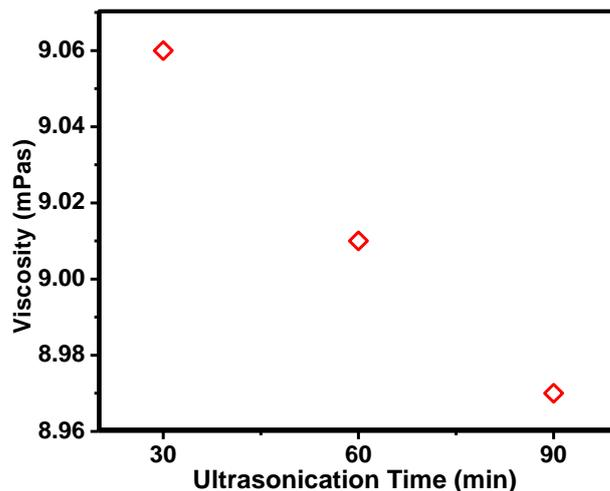
Figure 4. Variation of viscosity with ultrasonication time of ZrO<sub>2</sub>/H<sub>2</sub>O nanofluids.
