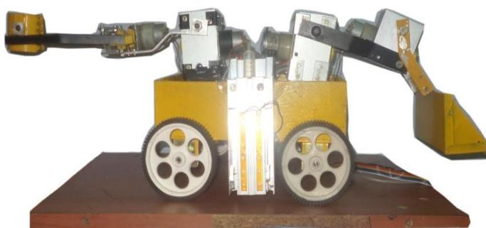
Figure 1. Multiple arms automated excavator
