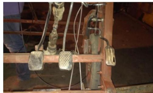
Figure 9.1 clutch,brake and accelerator
