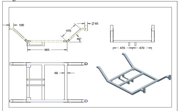
Figure1.1.The specifications of the frame
