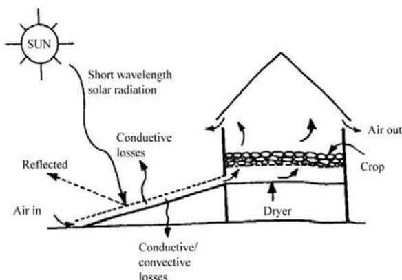
Working principle of indirect solar drying system (Sharma et al. 2009)[3]
