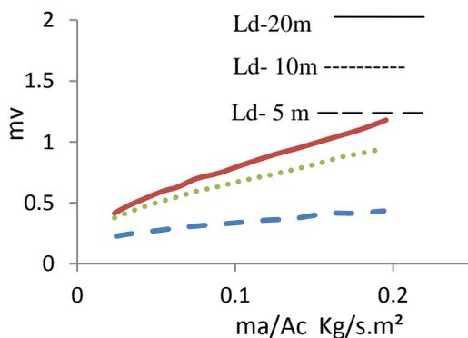
Fig.6. Vapour mass flow rate vs. hot air mass flow rate at drying chamber.
