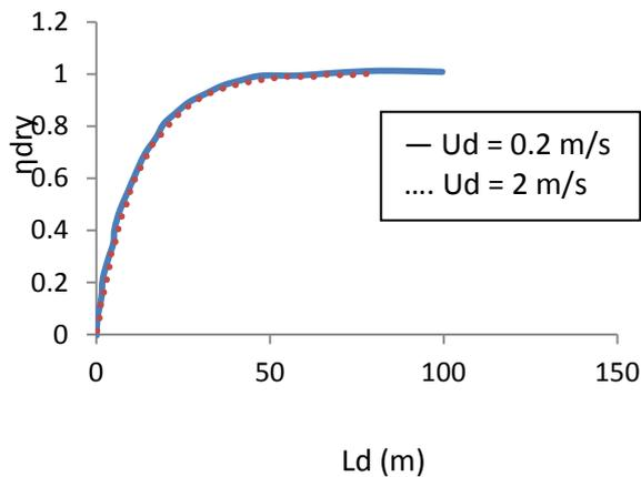
Fig.5. Drying efficiency along the length of drying chamber
