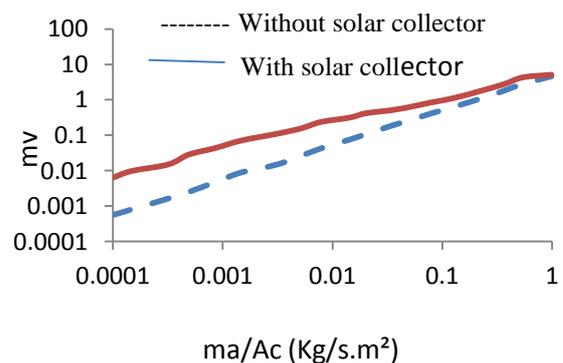
Fig.3. Maximum vapour mass flow rate with air mass flow per unit c/a of collector.
