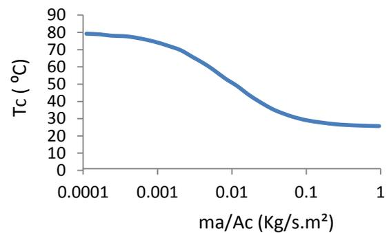
Fig.2. Temperature of air at collector outlet with mass flow rate.
