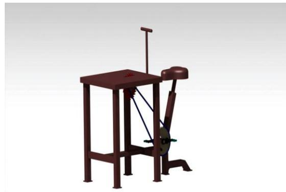
Figure 2. Human Powered Wood Cutting Machine
