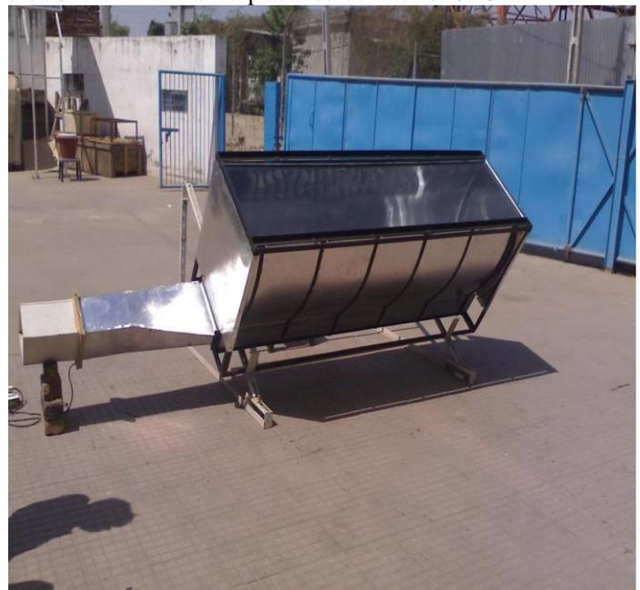
Figure 6. Picture to show the prototype of CPC Solar Air Collector.
