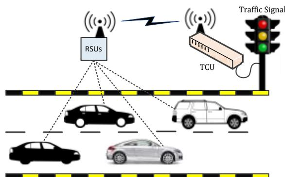
Fig. 4 Roadside Units Communication with Vehicles
