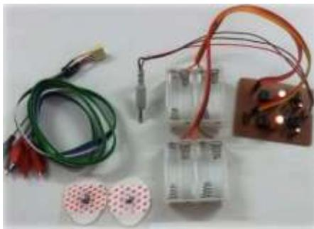
Fig. 4 Designed Stereo Amplification Circuit with Connecting Cables Which Is Responsible For the Amplification of Left and Right Movement of Eyes
