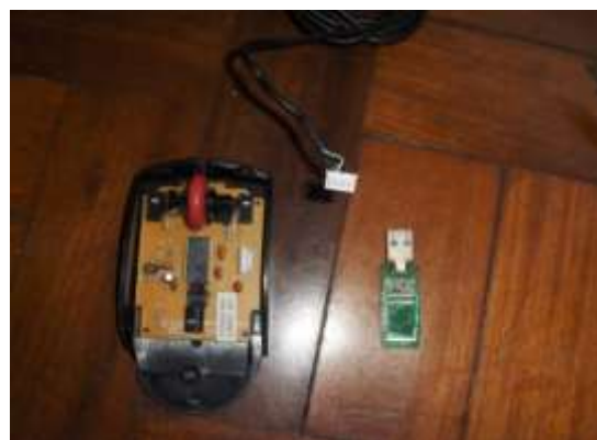
Fig. 5: USB dongle inside the Mouse for hidden storage for logs data.
