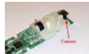
Figure 4. Wii Remote's IR camera
