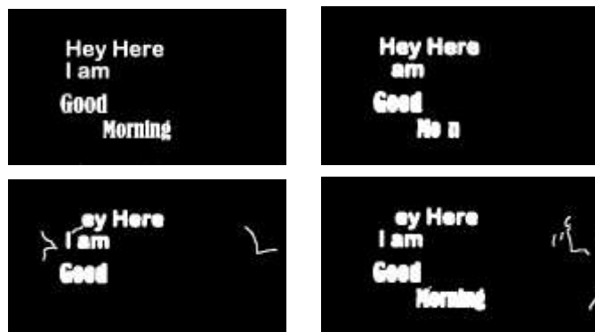
Fig. 2. Text Detection Results: (a) Actual Text existing in image, (b) Text Detected using Stroke Width Transformation, (c) Text Detection using Implemented method without Smoothing, (d) Text Detection using Implemented method with smoothing.
