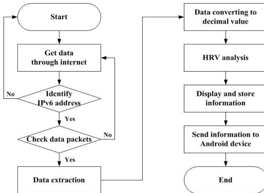
Fig. 2 Flowchart for data processing in the server
