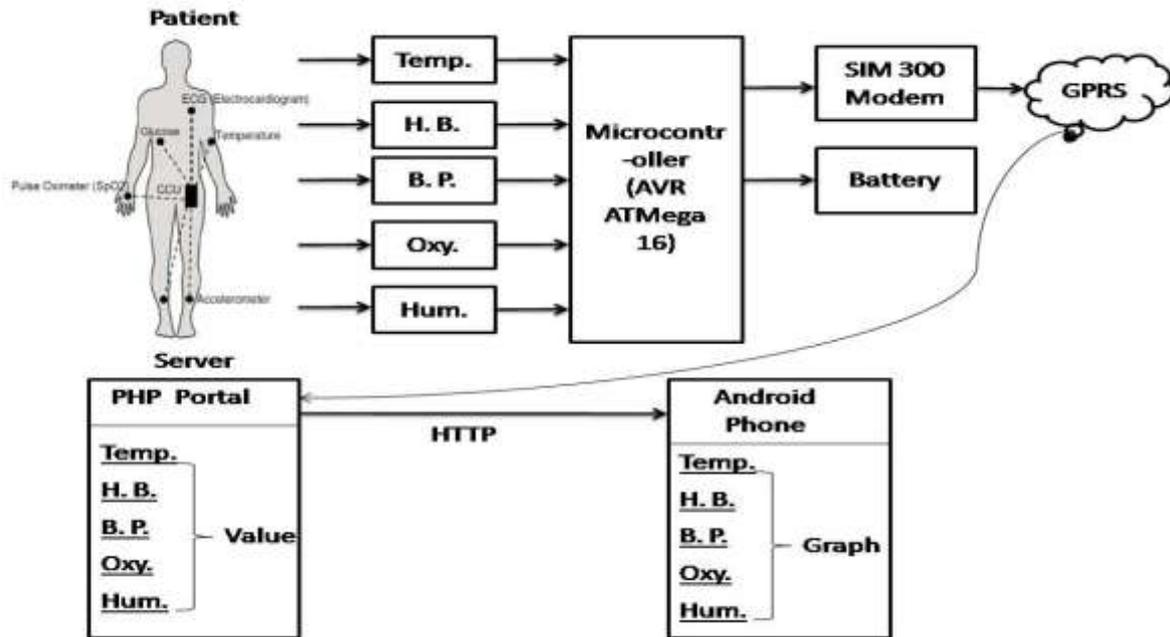
Fig.3. Block diagram of the proposed system architecture
