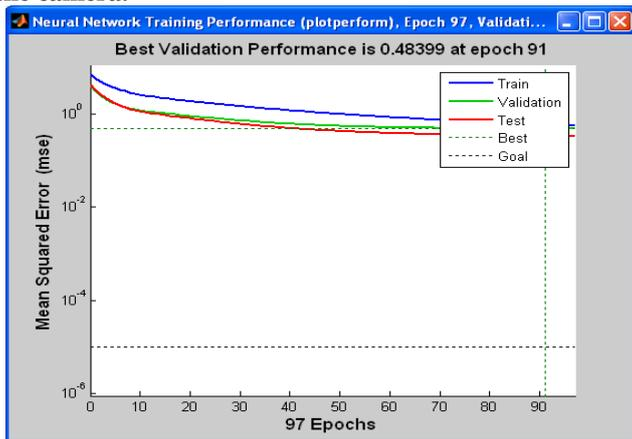
**Figure 10: Performance of Neural Network with gesture input in light environment at distance of 1 meter from the camera.**
