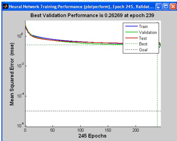
**Figure 9: Performance of Neural Network with gesture input dark environment at distance of 1 meter from the camera.**
