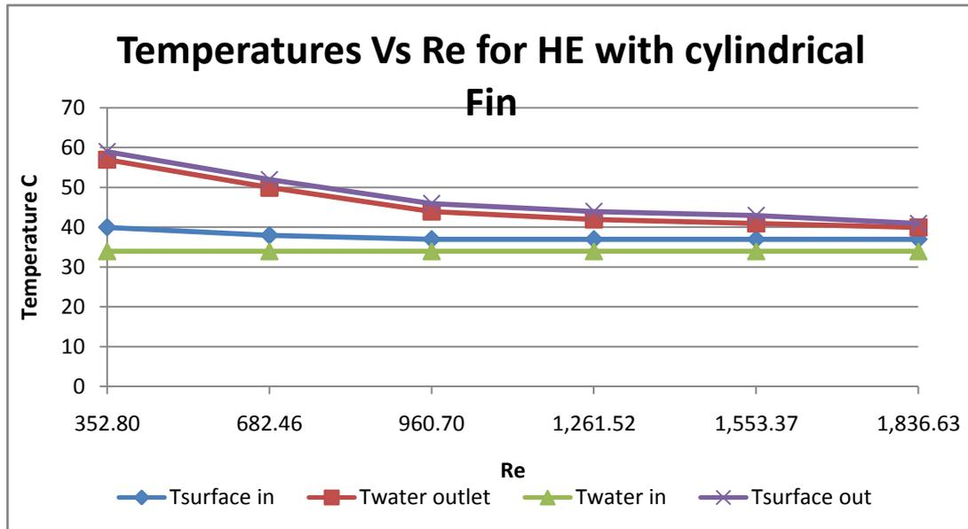
Figure 3 Variation in Temperatures with respected to Reynolds number for HE with Cyl. Fin.
