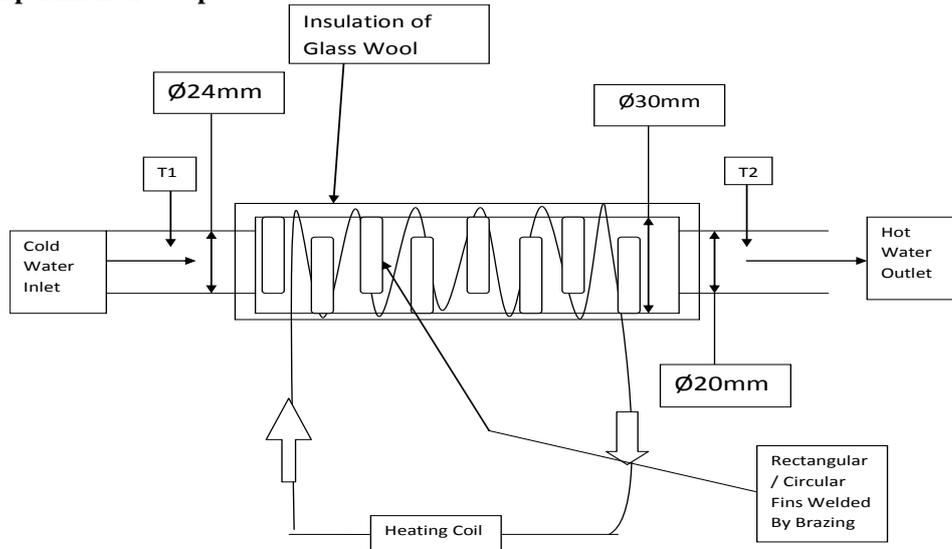
Fig.1 Line Diagram of Experimental Setup
