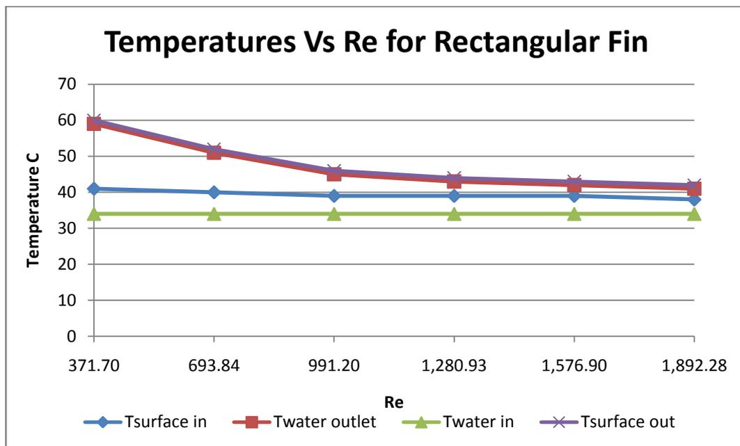
Figure 4 Variation in Temperatures with respected to Reynolds number for HE with Rect. Fin.
