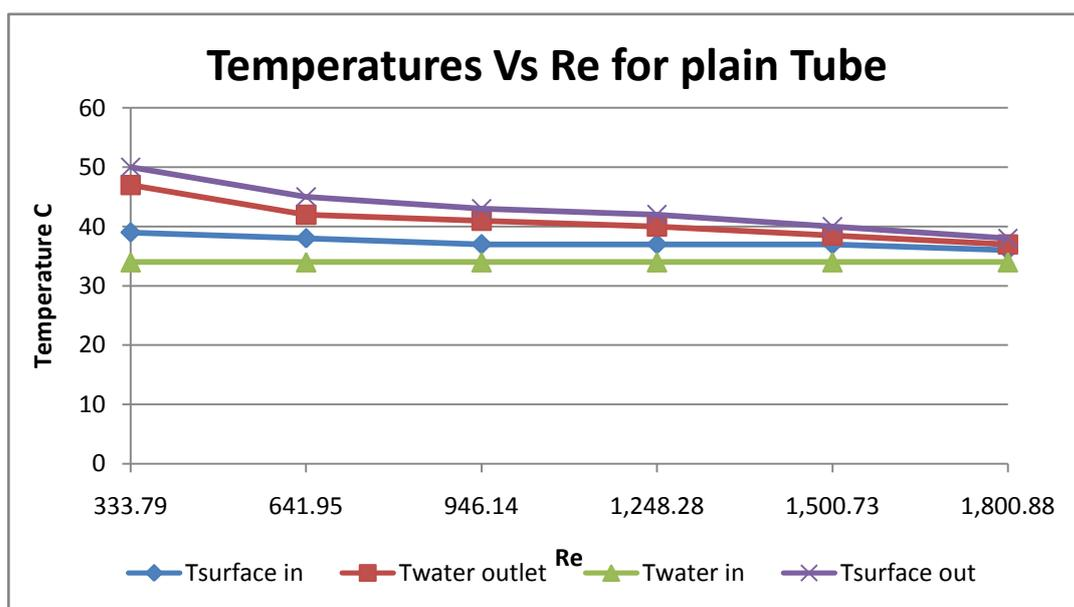
Figure 2 Variation in Temperatures with respected to Reynolds number for HE with Plain Tube.
