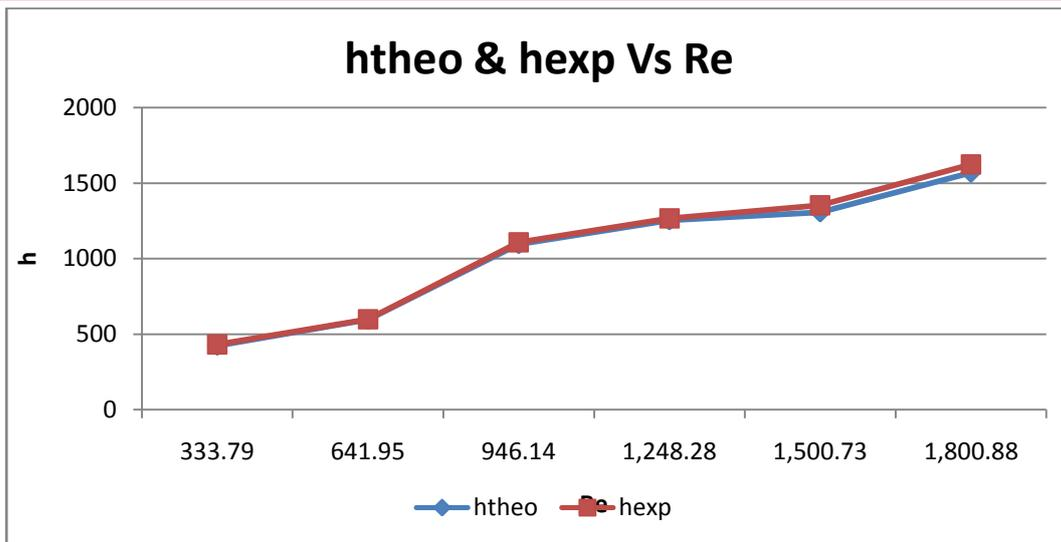
Figure 5 Variation in heat transfer co-eff. with respected to Reynolds number for HE plain Tube.
