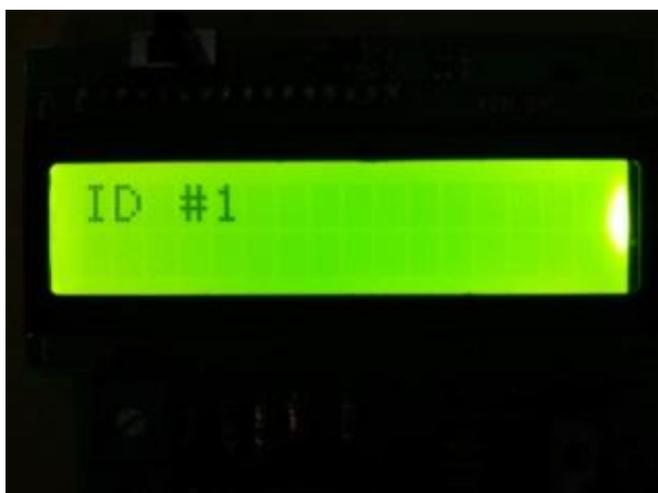
Fig 4: The device displaying the unique ID of a student when he/she places his/her finger on the fingerprint sensor
