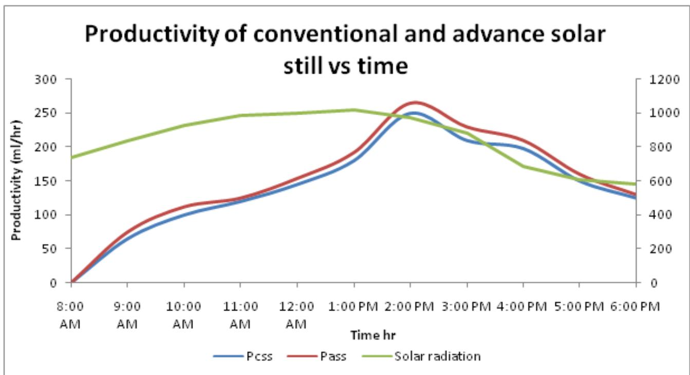
Figure 5 variations in productivity vs. time vs. solar radiation for 1cm water depth
