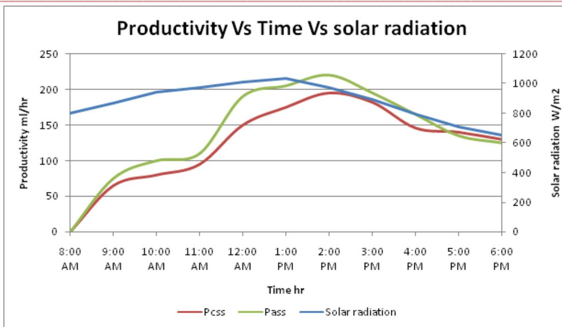
Figure 6 variations in productivity vs. time vs. solar radiation for 1.5cm water depth
