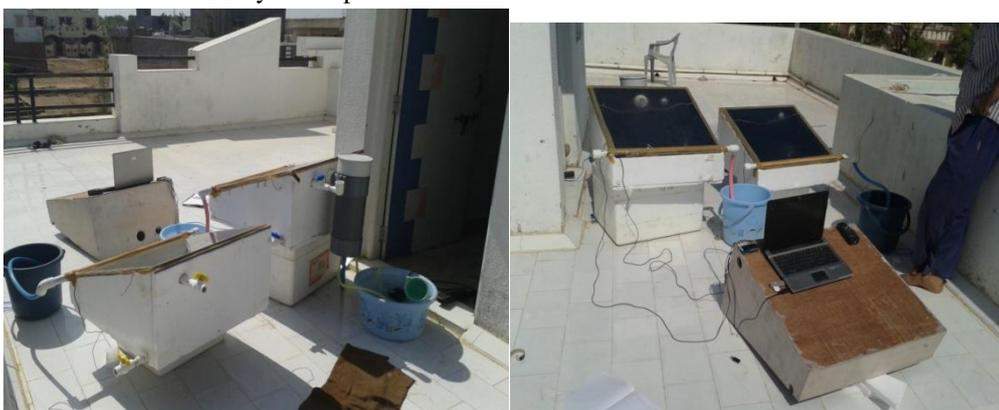
Figure 2 photographs of experimental set up with and without condenser solar still
