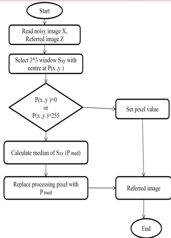
Figure-5 Flow graph of median filter
