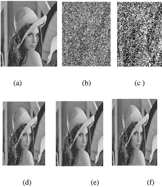
Figure-8. Results for 80% noise corrupted Lena image (a) original image (b) 80% noise corrupted image. Restoration results of (c) Simple median filter (d) Decision based median filter (e) Decision Based Unsymmetrical Trimmed Median Filter (f) Adaptive median filter
