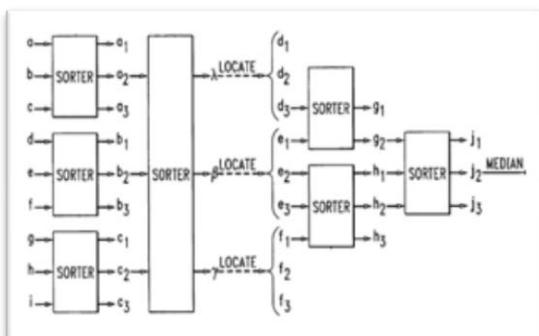
Figure-2 Architecture of median filter [8]
