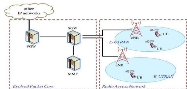
Fig-1 LTE system architecture
