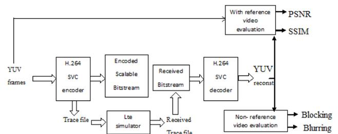
Fig. 3. Experimental setup to evaluate SVC video performance
