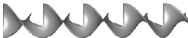
Fig. 7: Parabolic-cut twisted insert [7]
