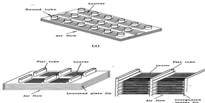
Fig.5 Typical fin-and-tube heat exchangers (From Wang et al., 1999) [4]
