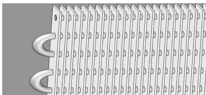
Fig.4. View of a single row fin-and-tube heat exchanger [3]
