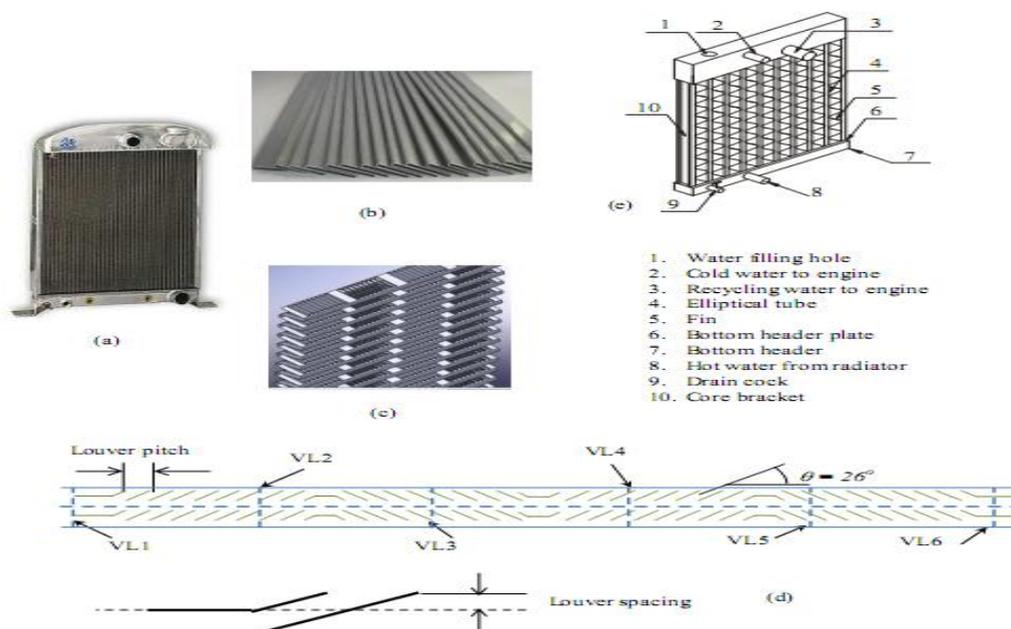
Fig.2. Details of radiator test unit [1]
