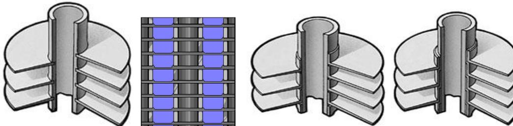
Fig. 1 Common Types of Fins Provided on the Tubular Heat Exchanger
