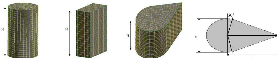
Fig.7. Studied morphologies: Cylindrical, Rectangular, and Drop-Shaped [5]
