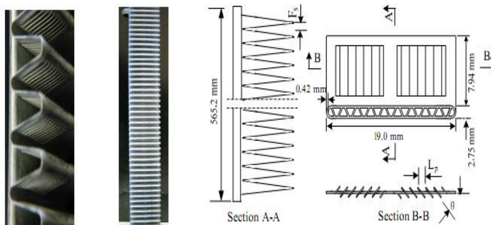
Fig.3. Structure of the test heat exchanger [2]
