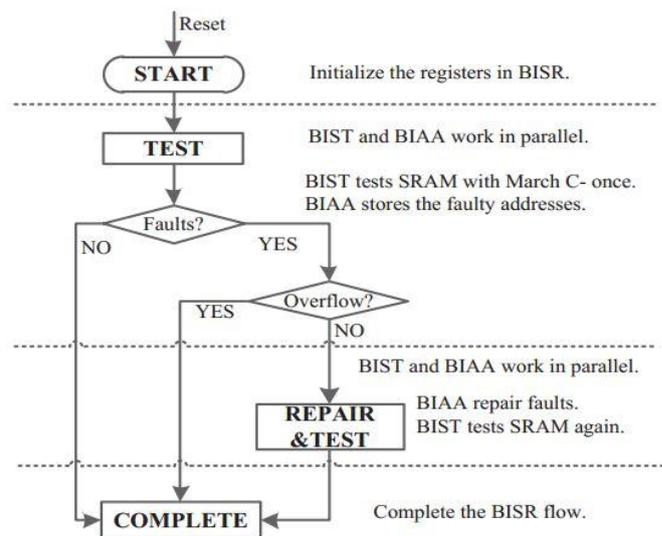
Figure 3: Block Diagram of BISR
