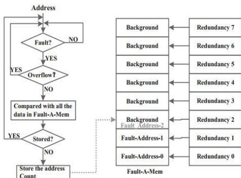
Figure 4: flows of storing fault address
