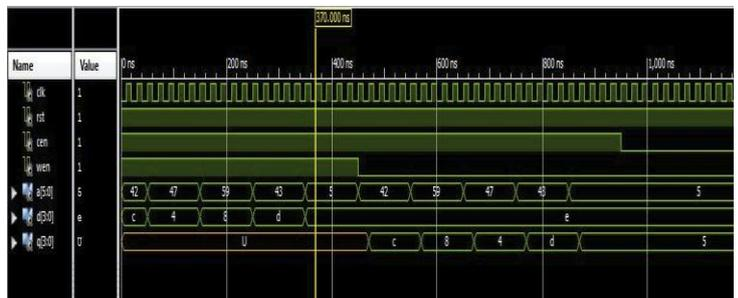
Figure 6: SRAM simulation
