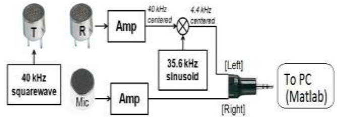
Fig-01 Ultrasonic Sensor circuit
