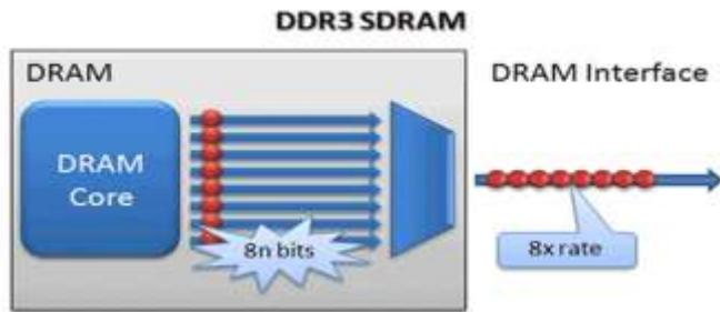
Figure 2: DDR3 SDRAM with 8-bit data rate
