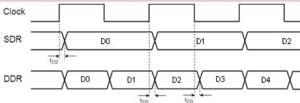
Figure 1: SDR and DDR timing diagram
