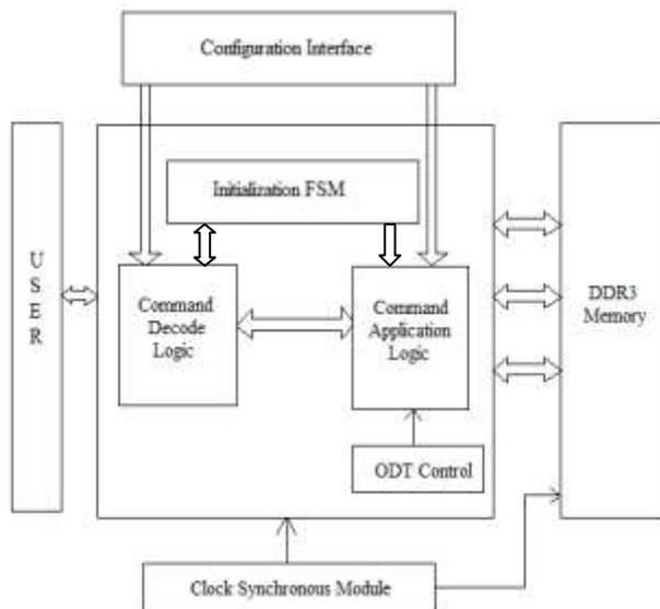
Figure 3: DDR3 SDRAM Controller Block Diagram
