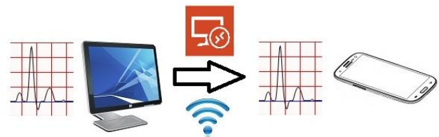
Figure 9. The Architecture of ECG Simulation Remote Desktop Connection.
