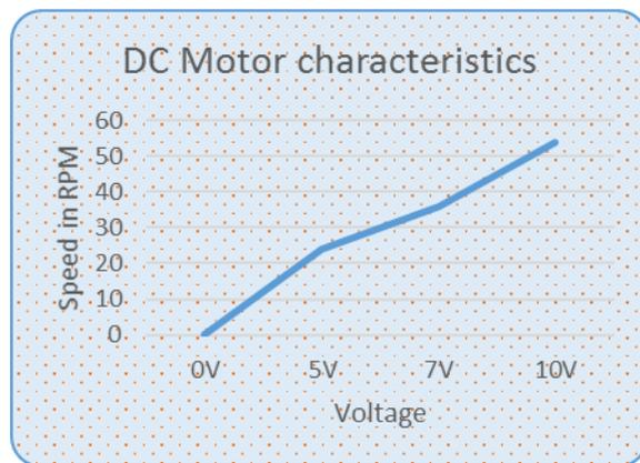
Figure 12 – Speed VS voltage characteristics of DC motor
