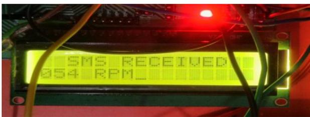
Figure 9 – Speed in RPM displayed on LCD display
