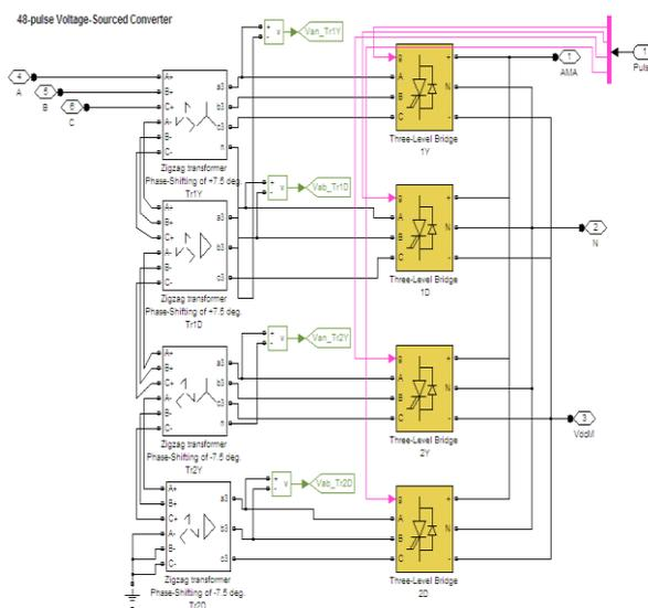
fig-2(48 pulse 3 level GTO based inverter)
